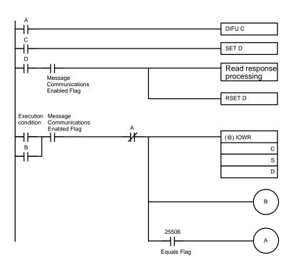
**Note** If the read response processing is executed after IOWR, there can be no Message Communications Enabled Flag response by means of IOWR, so an attempt could be made to read the response even though the message communications have not been completed.
